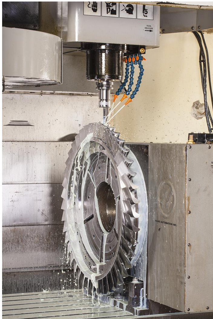
Nozzle Blades under Machining
